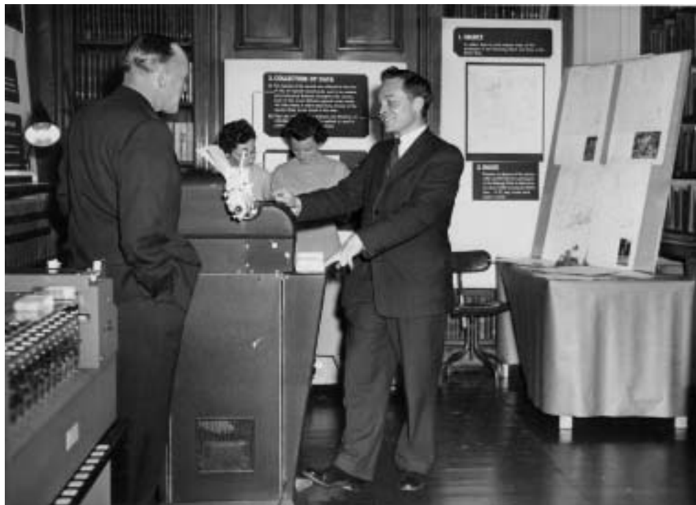
FIGURE 2. Frank Perring demonstrating the tabulator modified to print the maps for the Atlas of the British Flora .
